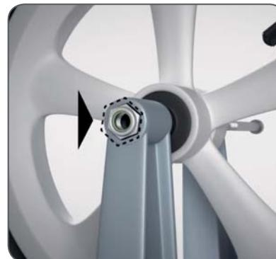
7. Insert the self-locking nut (Part F) into the hexagonal hole on the left side of the fork and insert and tighten the wheel bolt (Part E) from the right side using the hexagon (\"Allen\") wrench (Part G).
