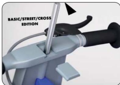
3. Hold the front fork and frame together at the headset groove and insert the headset axle (Part A), **threaded side on top**, into the headset. To ensure the headset axle (Part A) is inserted completely, the wheel bolt (Part D) may be placed on top of the headset axle (Part A) and gently tapped into place with a rubber mallet to avoid damaging parts.
