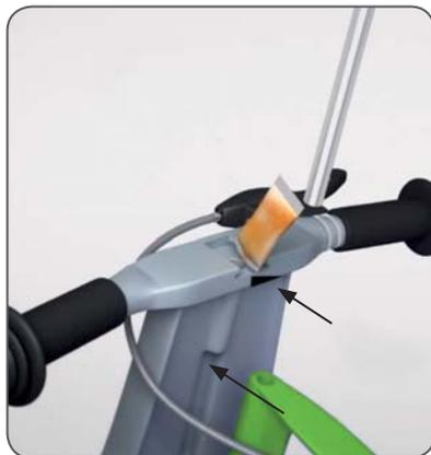
2. Open the lubricant (Part B) and lubricate the headset axle (Part A) and contact surfaces of the front fork and frame using 2-3 drops for each surface.
