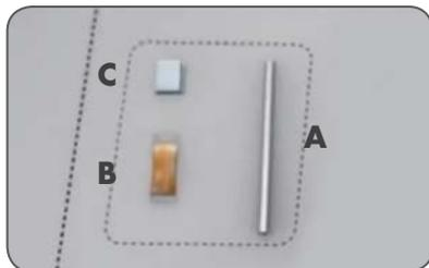
1. Open plastic bags containing headset axle (Part A), lubricant (Part B), and plastic cover (Part C).
