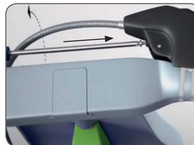
If necessary, adjust the brake cable tension with the adjustment screw located at the end of the brake cable by the rear wheel to ensure the brake does not rub or engage when the brake is not applied.
