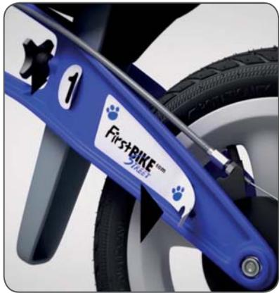
9. Apply adhesive stickers (Part G) according to the included Sticker Position photos. Note that the adhesive sticker for handlebar should be placed over the plastic cover (Part C).
