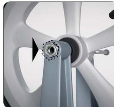
7. Insert the self-locking nut (Part E) into the hexagonal hole on the left side of the fork and insert and tighten the wheel bolt (Part D) from the right side using the hexagon ("Allen") wrench (Part F).
