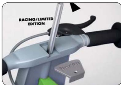
3. Hold the front fork and frame together at the headset groove and insert the headset axle (Part A), **threaded side on top**, into the headset. To ensure the headset axle (Part A) is inserted completely, the wheel bolt (Part E) may be placed on top of the headset axle (Part A) and gently tapped into place with a rubber mallet to avoid damaging parts.
