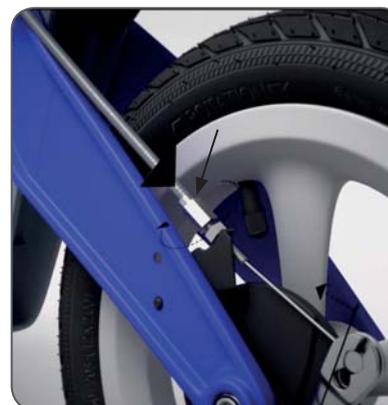
If necessary, adjust the brake cable tension with the adjustment screw located at the end of the brake cable by the rear wheel to ensure the brake does not rub or engage when the brake is not applied.
