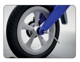
Use the hexagon ("Allen") wrench (Part E) to remove the rear wheel nut and bolt. If the bike is equipped with a brake, leave the brake plate attached to the wheel.
