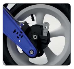
For FirstBIKE with a brake, ensure that the extruding black "pin" on the brake assembly is firmly inserted into the "upper" hole (from two holes) of the frame prior to tightening.
