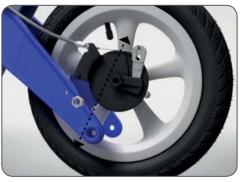
When the frame is separated from the rear-wheel assembly, allow the frame to drop downward in order to mount the left bracket (Part A) and right bracket (Part B).
