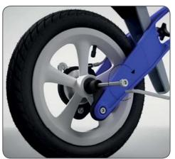
Tighten the rear wheel nut and bolt securely using the hexagon ("Allen") wrench (Part E).
