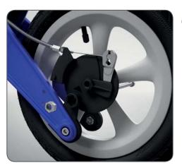
Once the brackets (Parts A and B) have been mounted on both inner sides of the frame, the rear wheel can be repositioned between the brackets (Parts A and B).
